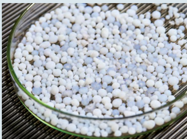
Little marvels: The aerogel is mixed into the plaster.
